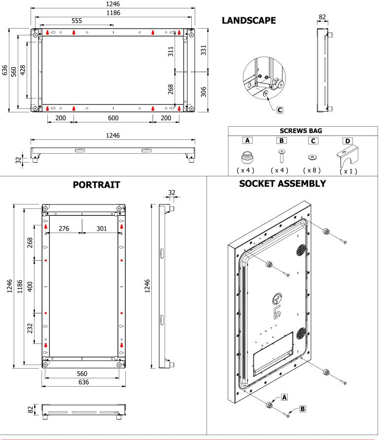
USE 4 HOLES ABOVE AND 4 HOLES BELOW FOR WALL FIXING (INDICATED IN RED).
